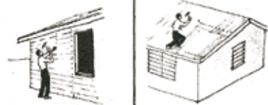
Hurricane preparedness: blocking gaps in the eaves and under shelters, securing walling and roofing sheets
