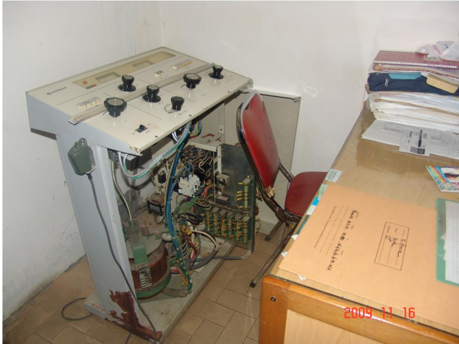
Damage to medical equipment, Selaguri hospital, Overturning and Damage to the X-ray equipment observed 2009 Ache earthquake (IIEES, 2009)
